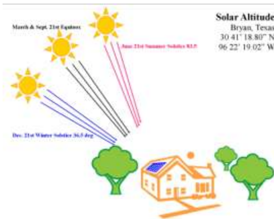
The solar altitude determines what angle the sun will rise and fall throughout the year.
