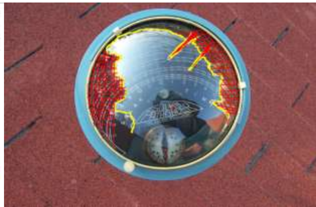
The Solar Pathfinder shows what areas of the site are obstructed by trees or other things that would prevent the full amount of sunlight from reaching the panels throughout the year as the sun changes its path.
