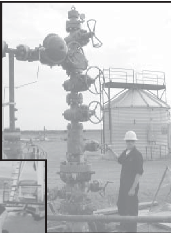
The assembly of wellhead and valves, often referred to as a Christmas tree.
