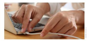
Unplug electrical appliances, especially equipment such as televisions, game consoles, and computers. These devices use power even when they are not on – known as 'phantom load'.
