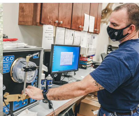
BTU Meter Technician Chris Stewart tests a digital meter for accuracy
