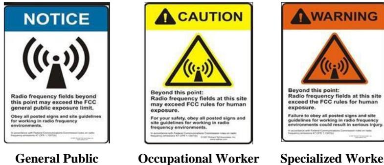
All signage shall be 8” x 12” and made of weather, corrosion, and ultra-violet (UV) resistant materials.
