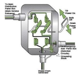
The DPDT transfer switch has three positions:
