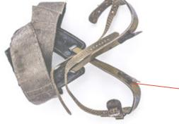
Steel points that enable linemen to securely climb poles. The only time we "hook 'em" around here is when linemen
